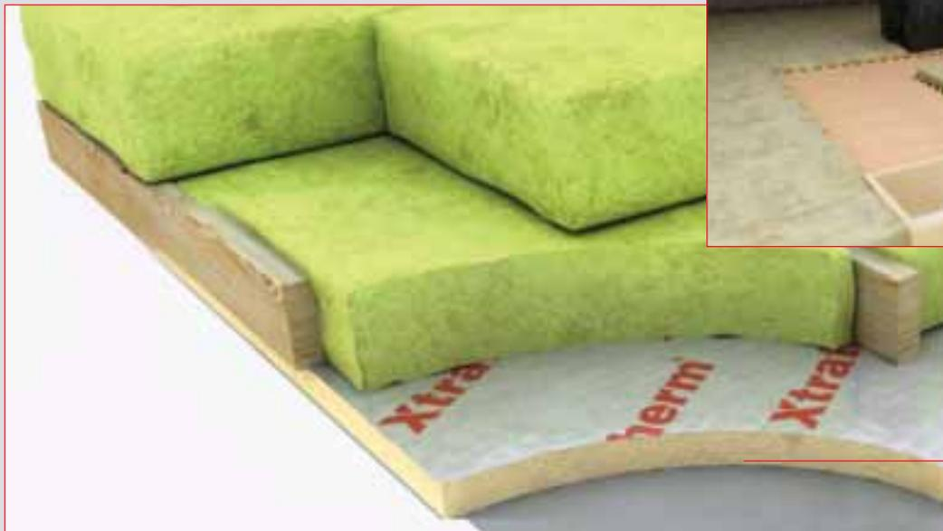
*Placing a layer of insulation to the underside of the ceiling will insulate the thermal bridging through the joists and allow the roof space to be floored (depending on joist depth)*
