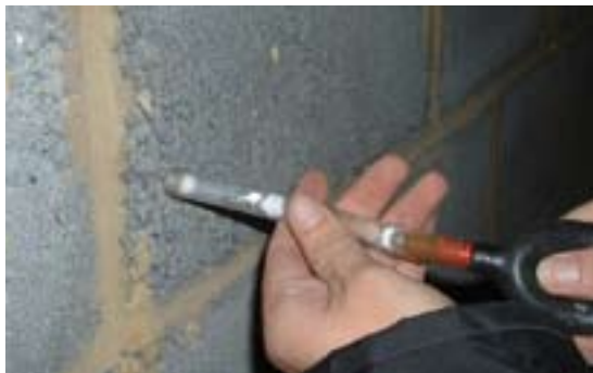
Figure 11 Air passing through porous concrete blocks
