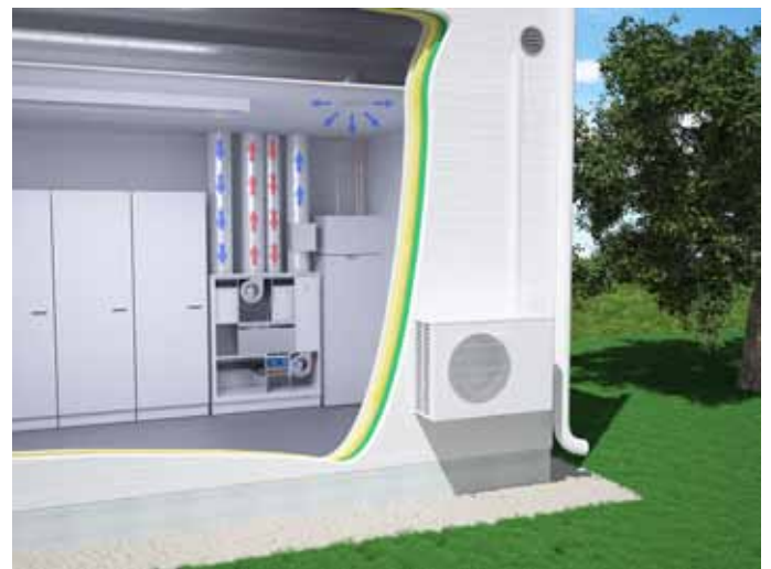
The air cooled by the EDX system heat pump is evenly distributed throughout the house using the ventilation ducts. Heat pump inside units aren't needed at all.
